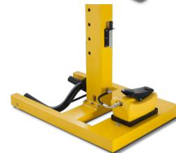
The UnoLiner LV3T Mobile Hydraulic Lift is a mobile hydraulic crick lift with a column structure, specifically designed to benefit its operator with its mobility and good working height. An air hydraulic pump, controlled by foot and connected to a strong chain, enables raising and lowering of the heavy-duty wheel fork or exchangeable sill clamp, which in turn raises and lowers one side of any vehicle up to 3 tons in weight with ease.
